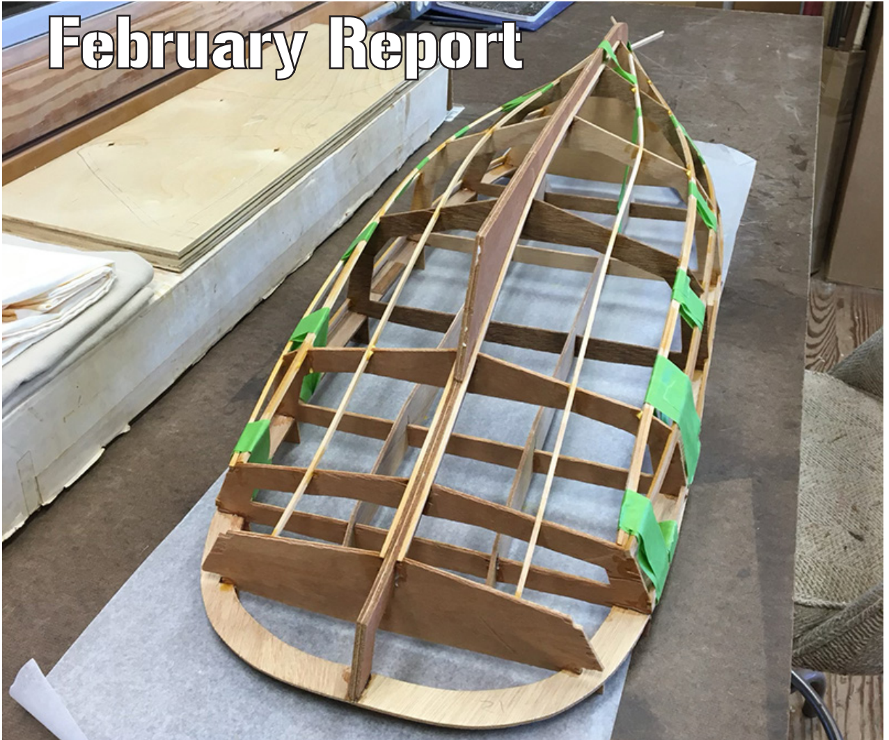
(above) Steve Michel's Harbor Tug frame resting easily on her main deck. This shows clearly the form she is taking.
