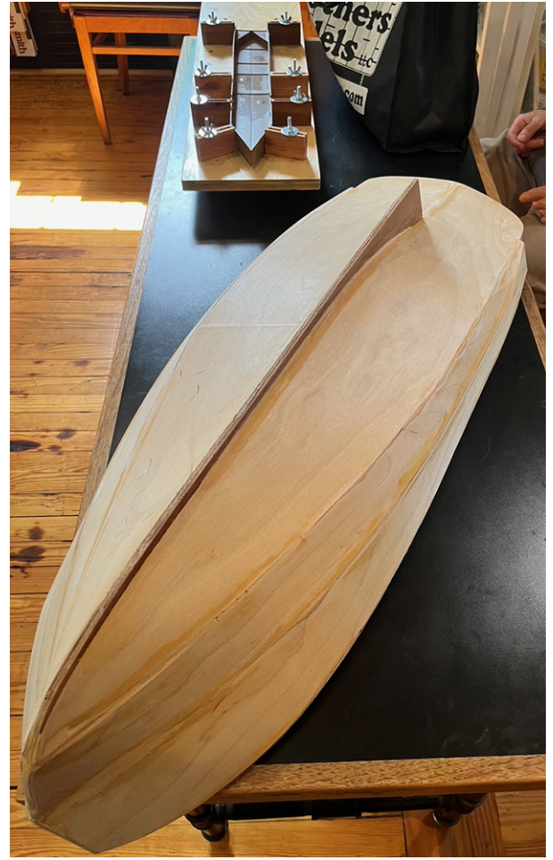
(above) shows the outer skin covering of the hull. Now the fun begins on sanding and filling and sanding and filling and a few bottles of that mountain elixir!
