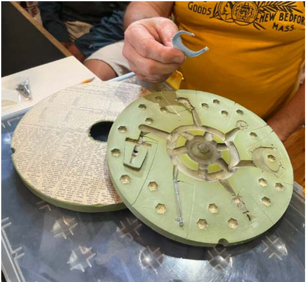
(above) A mold Denny uses for his spin casting technique.
