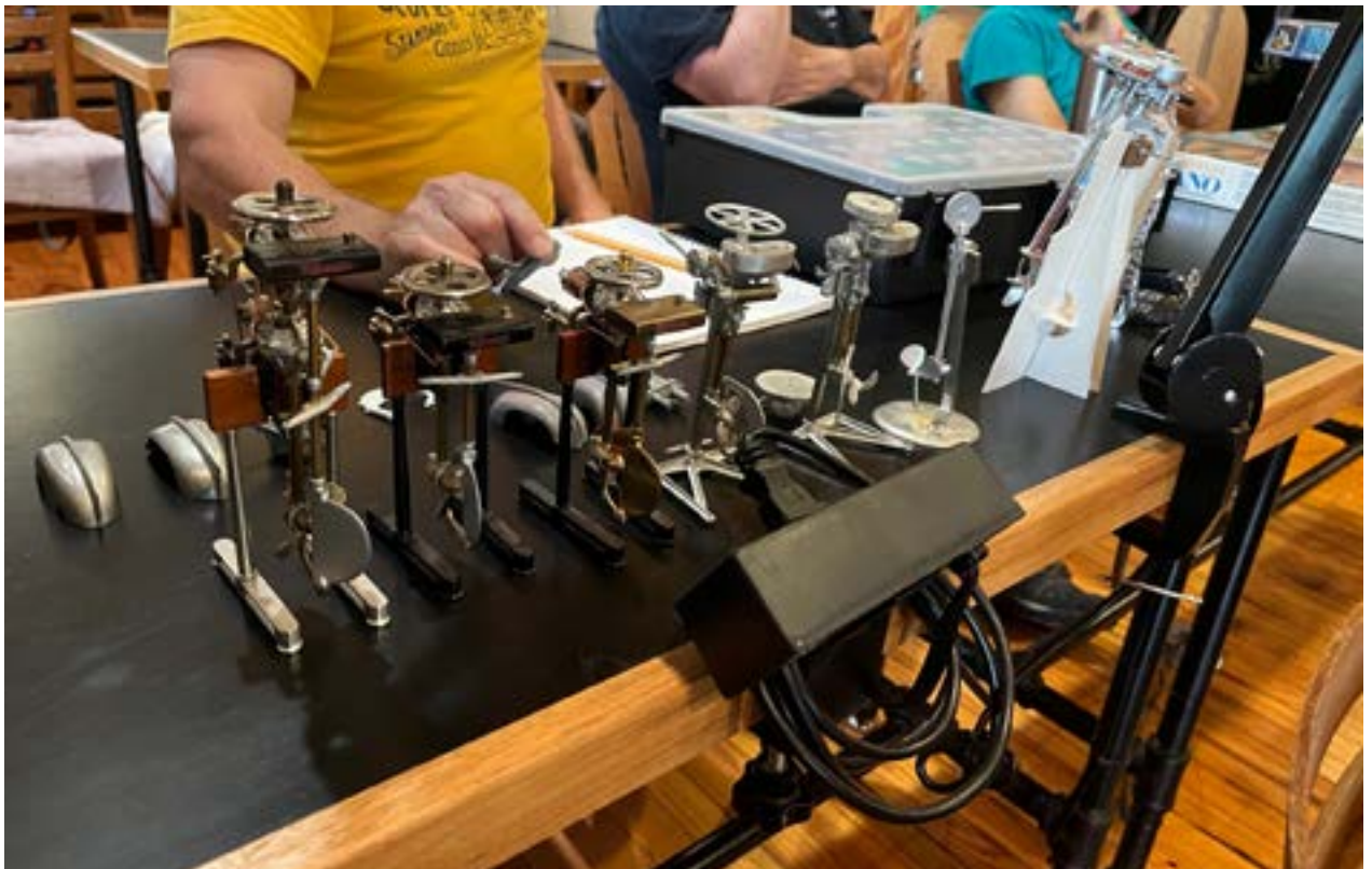
(above) Denny Cole’s motors displayed left to right: 1914 Waterman, 1914 Waterman, 1916 Koban, 1917 Koban, 1950 Men-U-Troll pump motor (the most interesting model) you hand pump the drive assembly which in turn, turns the prop. 1/8 scale, 1930 Elco Cub at ¼ scale and was on the market for a grand total of $26.50
